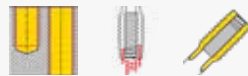
through holes & blind holes up to 2 x D Chip removal (like picture) Form C straight flutes
